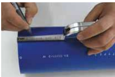
Measure and mark the pipe
